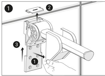
Gently remove the covers by lifting from the bottom. Remove the top cover and lift the arm off the bracket to get to the mounting plate.
