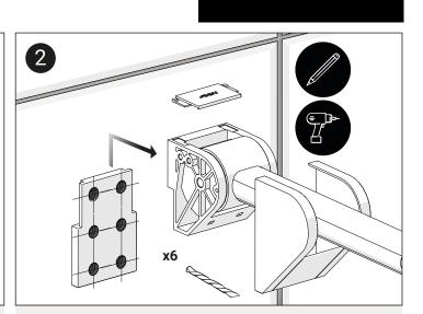
Mark out the desired height and mounting position using suitable tools. Drill the mounting holes.
