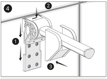
Attach the arm to the mounting plate. Reinstall covers.
