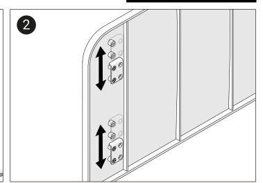
Further height adjustment can be made by adjusting the seat brackets on the backrest.
