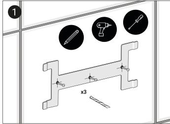
Remove bracket from the backrest. Mark out the desired height and position.
