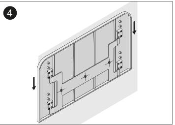
Slide down to attach to the mounting bracket.
