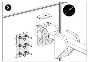
Fix the mounting plate to the wall using suitable wall fixings. Max 90kg load rating.
