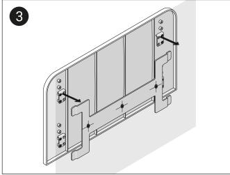
Align the backrest on to the mounting bracket.
